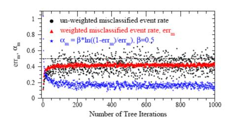
→ Boosted decision trees focus on the misclassified events which usually have high weights after hundreds of tree iterations. An individual tree has a very weak discriminating power; the weighted misclassified event rate err<sub>m</sub> is about 0.4-0.45.
