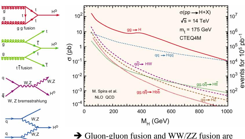
→ Gluon-gluon fusion and WW/ZZ fusion are two dominant Higgs production mechanism.
