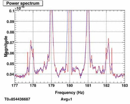
As we can infer from this plot, there must be some more sidebands between  $179 \sim 181$  HZ. For instance,  $180.0 \pm 0.2$  Hz are very likely to be a pair of sidebands. However, since 180 Hz move three times faster than 60.0 Hz, the 180 Hz peak is very wide. In fact this peak completely tops the
