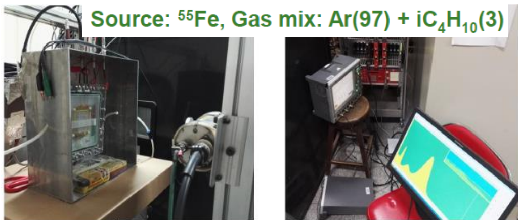
Photo of the GEM+Micromegas Module with X-ray
