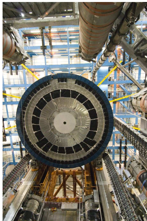
Figure 9.9: The end-cap calorimeter on side A in its fully open position with all three drag-chains and the flexible LAr fill-line connected.
