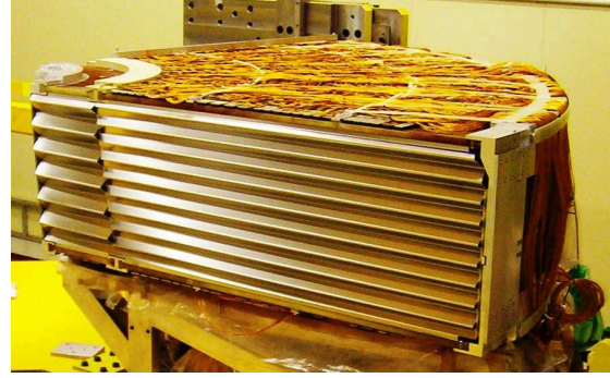
Figure 5.6: Photograph showing a side view of an electromagnetic end-cap LAr module (the beam axis is vertical). The first accordion absorber of each wheel is clearly visible, as well as the summing boards, the mother-boards and the cables.
