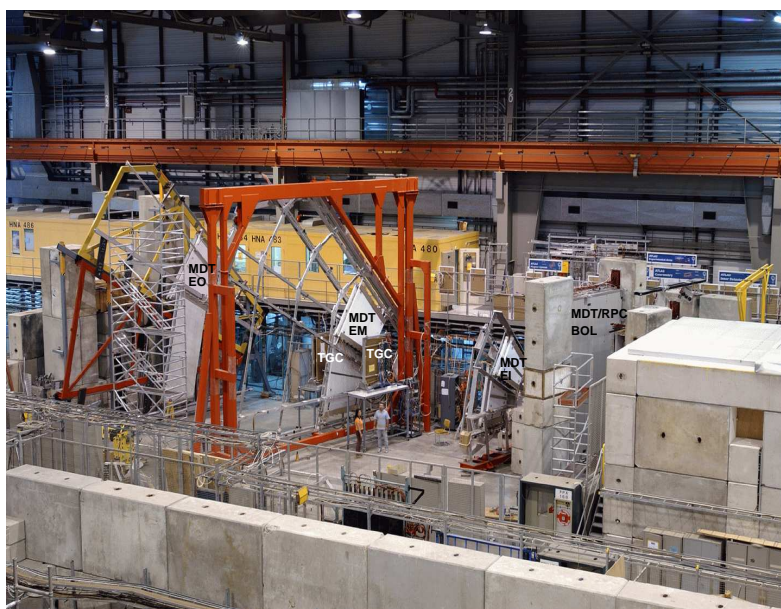
Figure 10.3: Picture of the combined test-beam set-up for the end-cap muon chamber system. The beam particles come from the right side of the picture, traverse the barrel muon chamber set-up, which is mostly hidden by the concrete blocks, and then go through three stations of end-cap MDT and TGC chambers.
